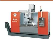
8 Vertical Machining Centers are available for tool making
